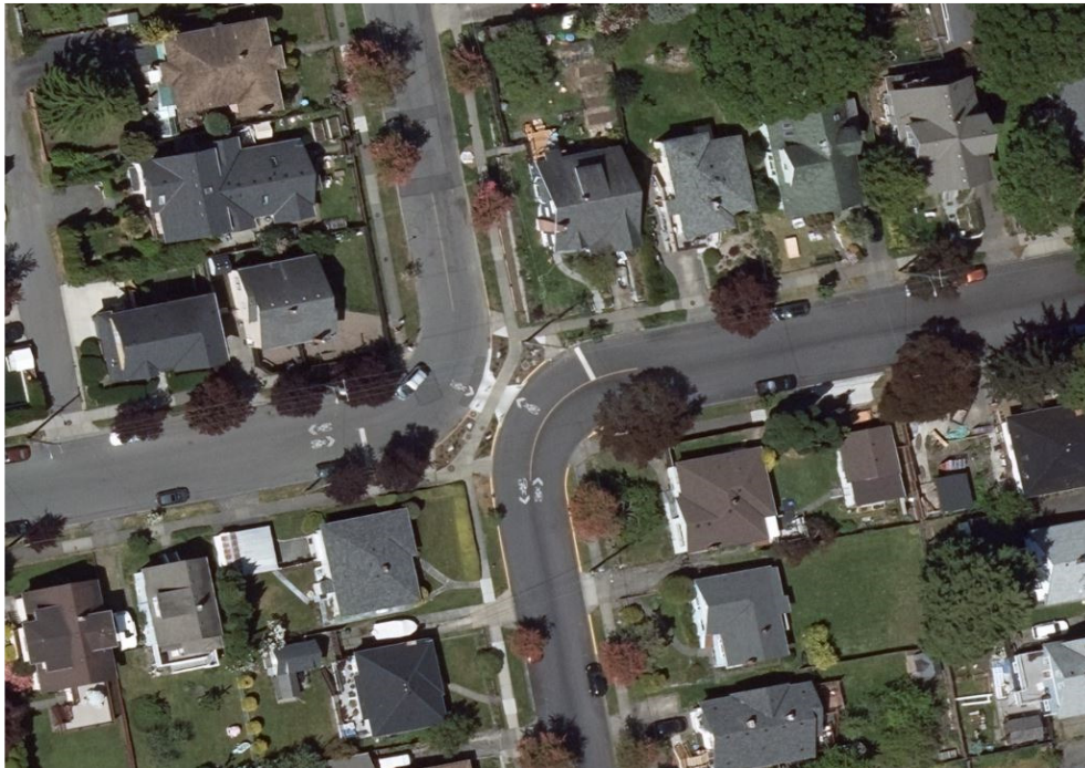
Diagonal Diverter at Blackwood St at Kings Rd, Victoria
